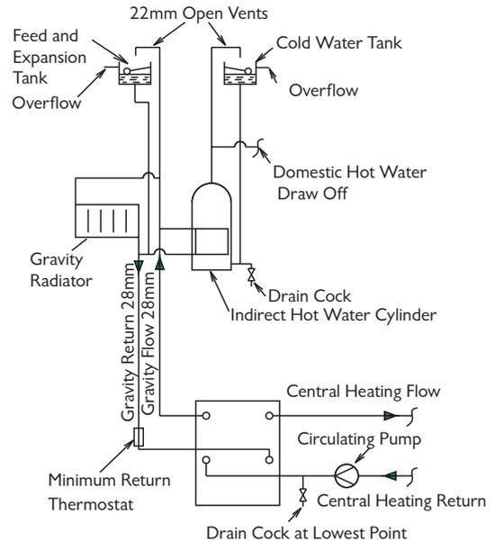
Fig. 7. Typical Central Heating & Hot Water System Using 3 Tappings
