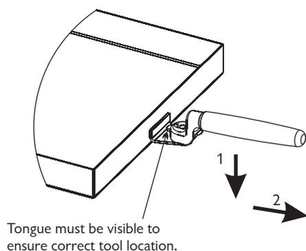
the slot in the top of the tool before lifting (See Fig.3). Care should be taken to ensure that ash is cool before emptying it into plastic liners or bins.
