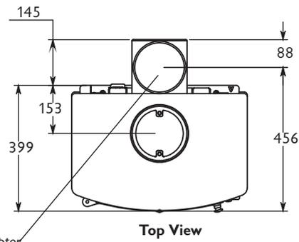
Flue outlet to suit 150mm (6" flue pipe)
