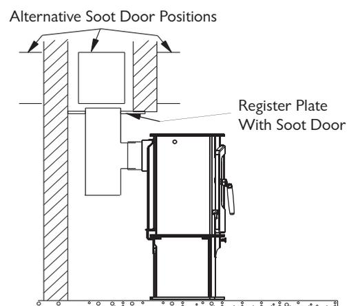
Fig. 11. Horizontal register plate with top flue connection
