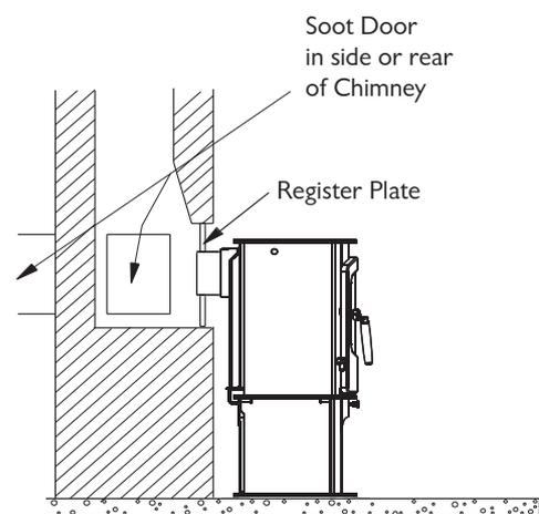
Fig. 10. Horizontal register plate with rear flue connection
